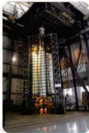
VLS – 1st Stage Separation Test Device
